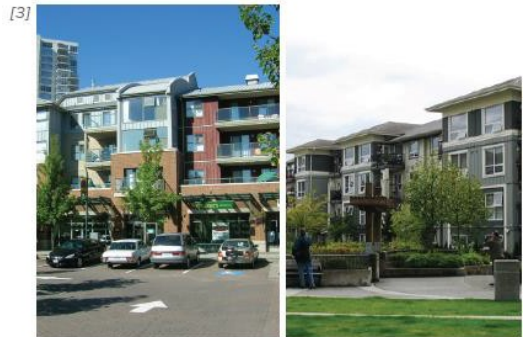
Large Building Elevation. [1] The front elevation of buildings with street-facing facades greater than 500 square feet should carve the building face into smaller, distinct planes, which can be accomplished by [2] incorporating a porch or dormer into the wall plan or [3] recessing the building a minimum of 2 feet over 6 feet.
