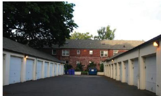
Street Facing Facade. [1] Attached garages on multi-dwelling units should not exceed 50% of the total building length as viewed from the street. [2] The maximum number of detached garages for attached or multi-family units is 4 attached garages that are a maximum of 24 feet wide each.
